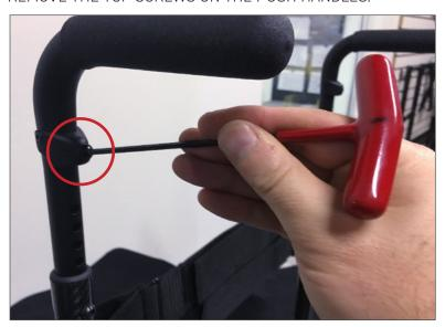
STEP 2 SLIDE THE STRAP WITH LARGE ENDS UP SO THAT YOU CAN SCREW THE PUSH HANDLE TO THE STRAP. REPEAT THIS STEP FOR THE OTHER SIDE.
