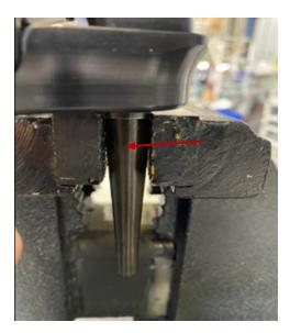
2. Put 1 drop of thread locker to the tip of the stem bolt and screw on the caster housing.
