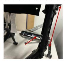
2. Screw back with the 26 mm socket and finalize the installation with the torque wrench adjusted to **61 Nm**.
