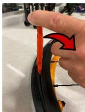
Press the tire out of the rim using the tire changer.
