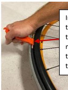
Insert the 2 sides of the tire into the rim using the tire changer, making sure that the tire is at the bottom of the rim.
