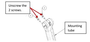
3. Use 1 of the 2 screws and insert it into the threaded hole located between the 2 screws to allow the clamp to open and move the mounting tube more easily to the desired location.
