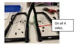
Join the connecting rods to the X-brace using the 2 screws (#91009) and a 3 mm Allen key.
