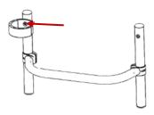
2. Put 1 drop of blue threadlocker on the tip of the screw and install the screw through the Velcro strap to secure it in place.
