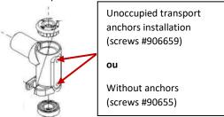
If there's an anchor, finalize the installation with the torque wrench adjusted to 7 Nm.
