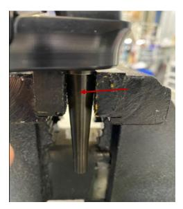
2. Put 1 drop of blue threadlocker to the tip of the stem bolt and screw on the caster housing.
