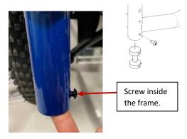
Put the eccentric inserts (#22080) on the screws (#4427) with the grooves on the same side as the screw head.
