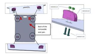
The top anchors (A and B) must be compatible with the clamps of the HELIO C2 H-Block supports. Move the H-Block seat support so that they are just in front anchors (A and B) to prevent the rigid seat pan to slide forward.
