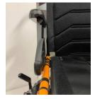
7. Finalize the installation with the torque wrench adjusted to 7 Nm.
