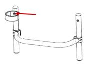
Put 1 drop of thread locker on the tip of the screw and install the screw through the Velcro strap to secure it in place.
