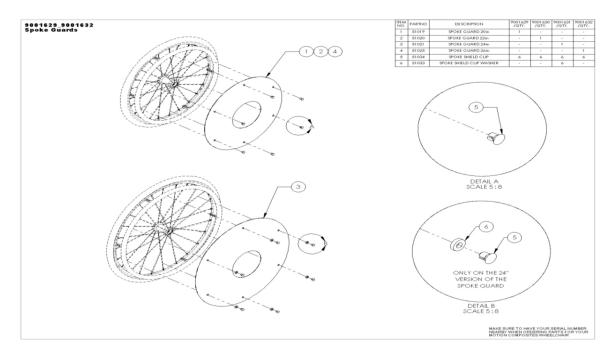
1. Fix the spoke guard on the wheel by hooking the clips on the spokes of the wheel.
