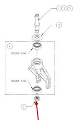
3. Tighten the nut (#7) using the 17 mm wrench.
