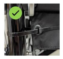
> Tighten, with the same tension, the left and right tie-wrap.
