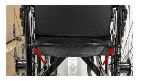
**2.** Cut the excess <u>as close as possible</u> to the fastener to void rubbing on the upholstery.
