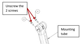
3. Use 1 of the 2 screws and insert it into the threaded hole located between the 2 screws to allow the clamp to open and move the mounting tube more easily to the desired location.
