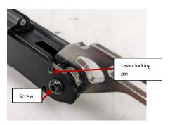
2. When the screw and the lever lock pin are removed, flip the lever over.
