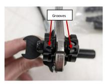
4. Replace the lever locking pin and the screws.
