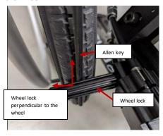
4. Tighten the 2 screws of the clamp on the frame and finalize the installation with the torque wrench adjusted to 7 Nm for a carbon frame and to 12 Nm on an aluminium frame.
