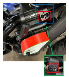
Make sure the wheel lock rod is <u>perpendicular</u> to the wheel.
