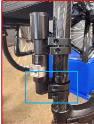
5. Before tightening everything, make sure the residual limb support is positioned at the desired distance. You can rotate the anchor as needed for optimal adjustment. Use the 4 mm Allen key.
