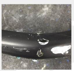
3. Use Isopropyl alcohol pad to remove pieces of tape that may remain on carbon and to clean it.
