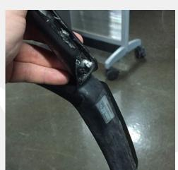
2. For the tape that still on carbon, you can easily remove the large majority by rolling the tape with thumbs.
