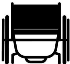
No camber angle or 0° camber or Zero camber
